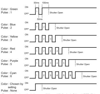
$\bullet$  The pulse signal must be in the range of 50ms  $\pm 10\%$  for both ON and OFF. IF the signal is out of this range, the input will not operate as a 50ms input.
